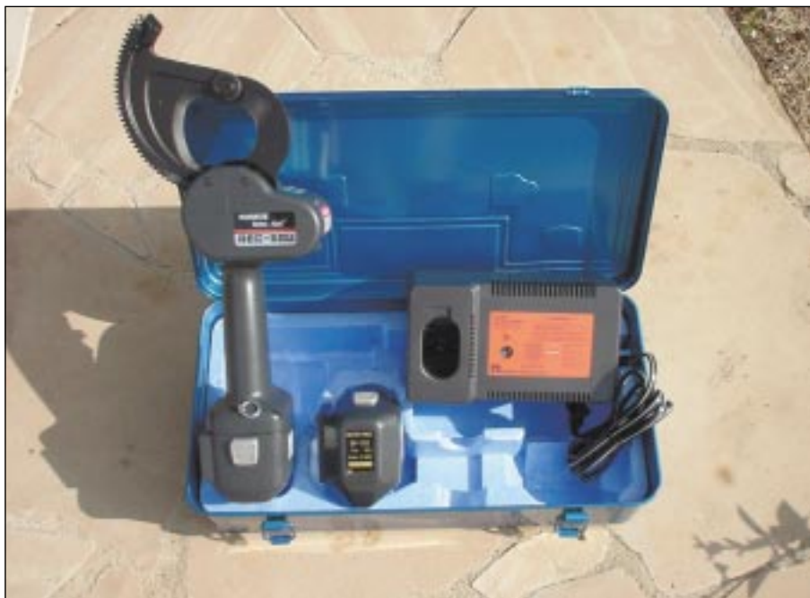
Figure 1 The OEL Wolverine robotic cable cutter represents the trend toward safer ergonomic tooling. Unlike conventional manual cable cutters, the stress of repetition for the installer is eliminated with only the touch of a button.
